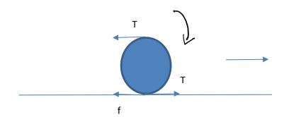
The diagram shows the front wheel subject to an anti-clockwise torque, but still rotating in a clockwise sense, and moving to the right.
