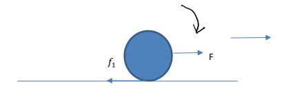
For the rear wheel, there is no torque from the engine, but the wheel is pulled along by the chassis, and friction  $f_1$  now acts to the left, to oppose the attempted motion.
