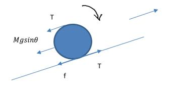
The diagram shows the front wheel. Supposing again that the frictional force acts down the slope:
