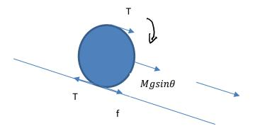
The diagram show the front wheel (assumed to be rolling rather than slipping). There are now two forces on the imaginary stationary block ( $T \& Mgsin\theta$ ), in opposing directions. Supposing for the moment that the frictional force acts down the slope:
