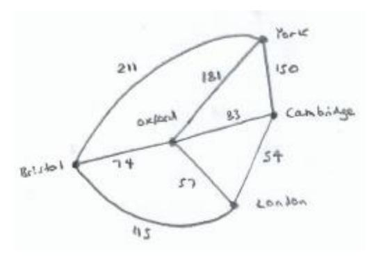
**Method 1:** Remove arcs in order of decreasing weight (ensuring that the network remains connected).
