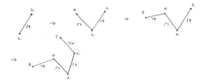
Method 4: Prim's Algorithm using the matrix of weights
