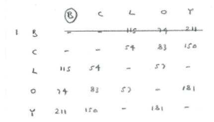
We then find the smallest weight in column B: 74 for O (indicating that O is the nearest node to B). We then circle this 74, for future reference, circle O at the top (to indicate that O belongs to the nodes selected so far), and cross out the row for O (to indicate that we no longer need any arcs that end in O).
