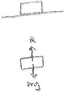
Drawing a force diagram for the object, and applying Newton's 2nd law gives:  $R = mg$ . Then, by Newton's 3rd law, the reaction force on the surface from the object is  $R$ , which we have found to equal  $mg$ .
