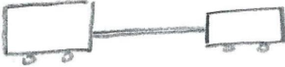
Assuming that the car is pulling on the towbar with a force  $T_1$ , then the towbar will be pulling on the car with the same force, by Newton's 3rd law (ie the car will experience a drag on it from the caravan, via the towbar).
