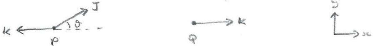
The impulse-momentum equation can be applied to 'impulse diagrams'.
