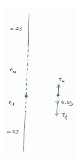
(i) Let the extensions of the upper and lower parts of the string be  $e_u$  and  $e_l$ , respectively, and the tensions in the two parts  $T_u$  and  $T_l$ .
