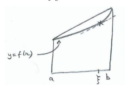
The diagram demonstrates this: the gradient of the curve at  $x = \xi$ , ie  $f'(\xi)$  equals the gradient of the line (ie  $\frac{f(b)-f(a)}{b-a}$ ).
