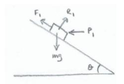
In the first case, resolving forces perpendicular to the slope,
