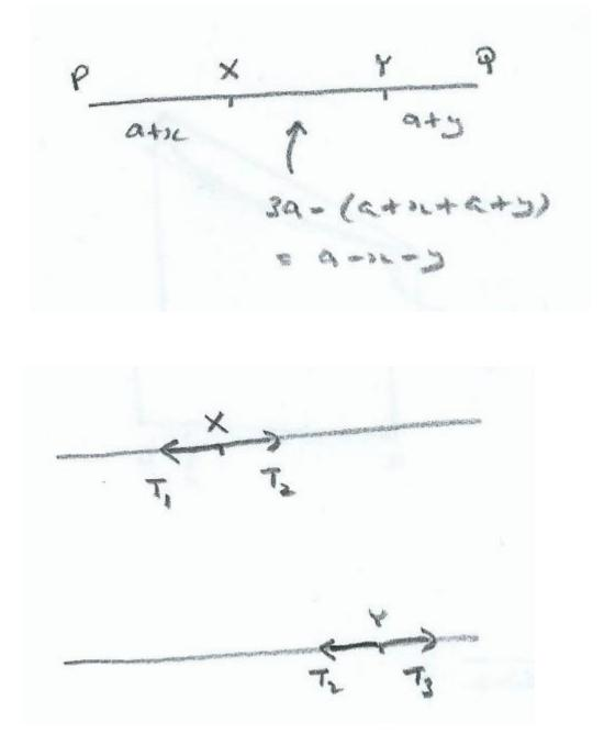
Referring to the diagrams,  $T_1 = \frac{\lambda x}{a}$ ,  $T_2 = -\frac{\lambda(x+y)}{a} \& T_3 = \frac{\lambda y}{a}$ , by Hooke's law (thus  $T_2 < 0$  and the force is a compression).
