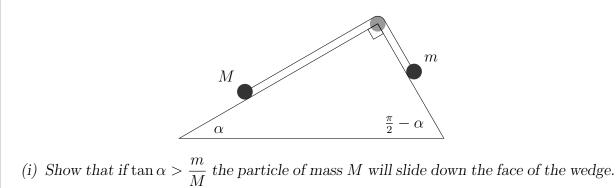
We start by drawing the forces on the picture, and labelling the masses as A (of mass M) and B (of mass m). We let T be the tension in the string.
