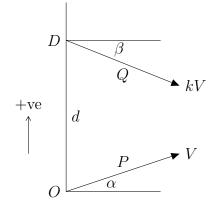
For components, we will write  $u_P$  and  $u_Q$  for the horizontal components of the velocities of P and Q respectively, and  $v_P$  and  $v_Q$  for the vertical components (measured upwards). For the displacements from O, we write  $x_P$  and  $x_Q$  for the horizontal components and  $y_P$ and  $y_Q$  for the vertical components.
