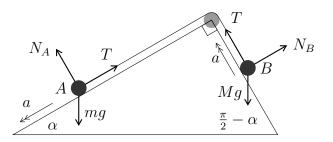
We now resolve along the faces of the wedge at A and B. (It turns out that resolving normally to the face doesn't help at all for this problem.)
