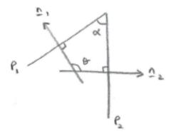
For the configuration of the normals shown in the diagram, the angle obtained from their scalar product ( $\theta$ ) is obtuse. In this case,  $\alpha = 180 - \theta$ . If either of the normals is reversed in direction, then the angle obtained from the scalar product is acute, and  $\theta$  in the diagram is obtained by subtracting the scalar product angle from 180. In this case,  $\alpha$  equals the scalar product angle. (If both
