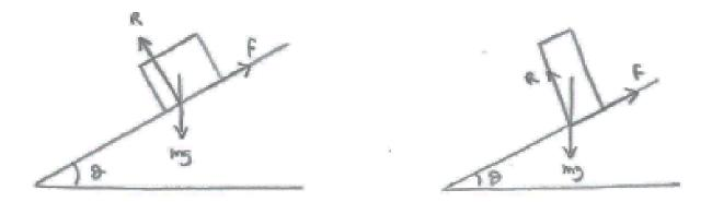
Whenever there are 3 forces on an object that is in rotational equilibrium, the lines of action of these forces must meet at a common point (otherwise the moment of one of the forces about the intersection of the lines of action of the other two forces would not be zero).
