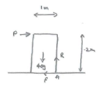
When the block is about to topple, it will be pivoting about A, so that R must act at A (as this is the only point of contact between the block and the surface). As the block is not yet rotating, the total moment about A must be zero.
