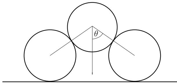
The weight of each disc is  $W$ . The coefficient of friction between a disc and the horizontal surface is  $\mu$  and the coefficient of friction between the discs is also  $\mu$ .
