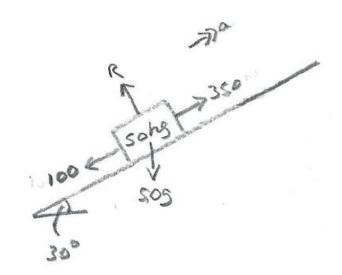
Resolving parallel to the slope and applying N2L:
