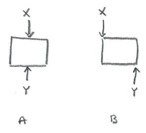
If the forces applied to an object are not liable to cause it to rotate (as in diagram A), then the object may usefully be modelled as a
