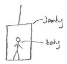
**Example 1:** The lift is accelerating upwards at  $0.5 ms^{-2}$
