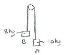
In the case of two blocks on either side of a pulley (as in the diagram), we cannot treat the two blocks and the connecting rope as a single object, as they are not moving in the same direction.
