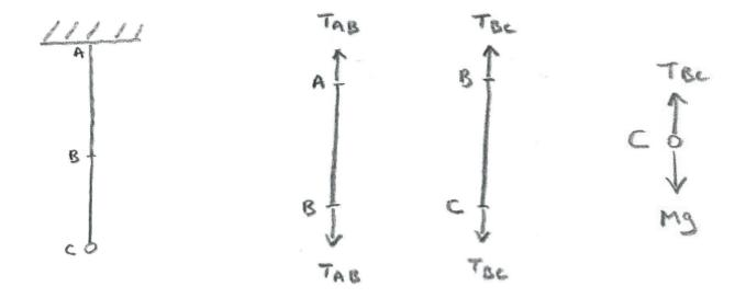
AB is in tension, and the forces at each end can be taken to be the same, because the string will be assumed to have negligible mass. To see this, suppose that the forces are  $T_A$  and  $T_B$ . Then, by N2L,
