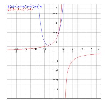
$1 + x + x^2$  is close to f(x) in a small interval around x = 0, and successive approximations get closer to f(x) for increasingly wider intervals of x
