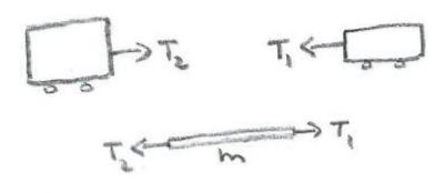
Applying Newton's 2nd law to the towbar, assumed to be of mass  $m, T_1 - T_2 = ma$ , where a is the acceleration of the car, caravan and towbar.
