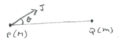
The impulse J has a component acting along PQ, and so the rod is under an impulsive thrust (of K, say), and by Newton's 3rd law, the rod exerts an impulse K on P.
