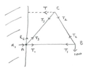
The convention for the internal forces is for inward-pointing arrows to denote a tension. The arrows are in effect the forces exerted by the rod <u>on</u> the joint (then, by Newton's 3rd law, the forces exerted on the rod by the joints are directed outwards; ie the rod is being pulled at each end, and is therefore under tension).
