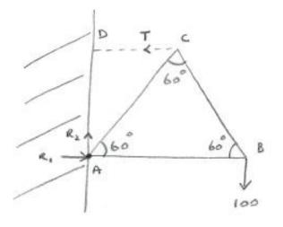
For framework questions, it is not usually worthwhile drawing separate force diagrams for each object (ie the joints A, B and C here). The above diagram shows the external forces on the framework, with the internal forces added in below.
