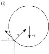
If the angle between mg and N is  $\theta$ , then conserving energy and either differentiating the energy equation or taking moments about the point of contact yields
